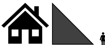
4. With your measuring tape, measure the distance from you to the base of the house. Because you were standing at a corner on a  $45^\circ$  right triangle, this is also the distance up the side of the house!
